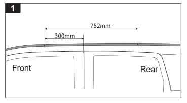
Roof ditch moulding requires holes to expose the roof rack fixing points. Mark points at measurements shown above.
