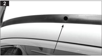
Front left hole position shown. Remove roof ditch mould.
