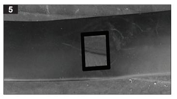
Cut hole's in each roof ditch mould approximately 12 mm square or with enough clearance to fit over the stud as shown in Step 6.
