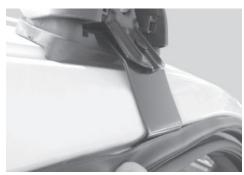
Open door. Pull rubber seal down. Fit clamp.
