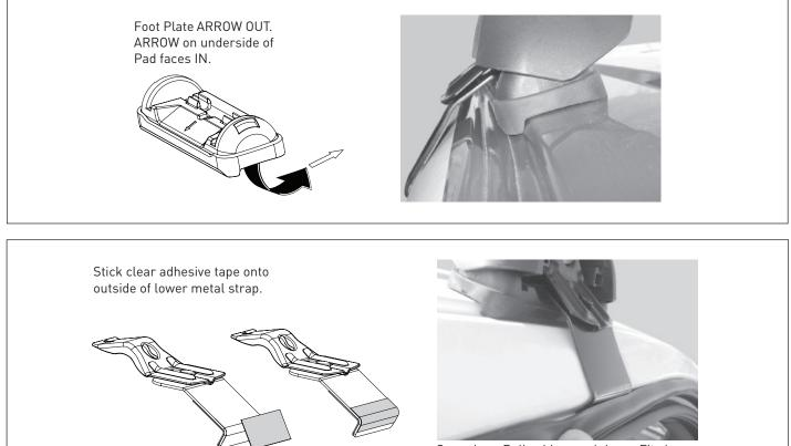
Open door. Pull rubber seal down. Fit clamp.
