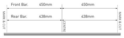
Note for dealers when altering a RSP kits: Add 38mm to sports bar measurement for RVL. Add 40mm to sports bar measurement for RVH.
