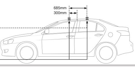
Note Vortex crossbars can be cut to length to fit this vehicle. Measure the desired length out from the centre of the Vortex Bar and create a reference with a marker. Carefully cut the bar at these markings using a Saw with an Alloy Cutting Blade.
