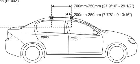
Note Vortex crossbars can be cut to length to fit this vehicle. Measure the desired length out **from the centre of the Vortex Bar** and create a reference with a marker. Carefully cut the bar at these markings using a Saw with an Alloy Cutting Blade.
