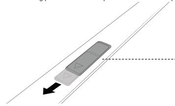
The mounting points will be exposed when the cover plates are removed.
