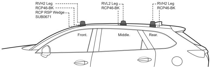
Note Vortex crossbars can be cut to length to fit this vehicle. Measure the desired length out **from the centre** of the Vortex Bar and create a reference with a marker. Carefully cut the bar at these markings using a Saw with an Alloy Cutting Blade.
