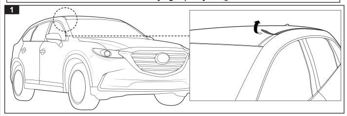
Locate the mount point brackets in the roof ditch. Screw in fixed mount studs as shown. Note: For a 2 bar system, use front and middle mounts only.
