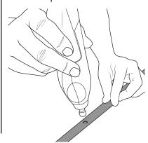
Replace the ditch mould. The studs will poke through the holes drilled in the mould.
