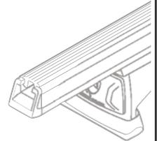
**Note** Vortex crossbars can be cut to length to fit this vehicle. Measure the desired length out **from the centre of the Vortex Bar** and create a reference with a marker. Carefully cut the bar at these markings using a Saw with an Alloy Cutting Blade.
