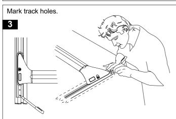
Remove rack from vehicle and crossbars from tracks. Drill holes using a 5mm drill bit. A drill stop is recommended to prevent drilling through roof lining. Vacuum vehicle roof to remove metal filings. Remove masking tape.
