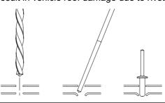
Apply cold galvanising paint around holes, once dry apply Selleys Butyl Mastic. Remove paper gasket from foam tape on underside of track. Locate track end caps, place tracks onto vehicle roof and rivet as shown.
