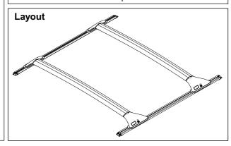
Locate legs into crossbar, use rubber mallet if required. Assemble rack as shown, attaching the legs to the tracks. Note: There is a left and right leg and spacer.
