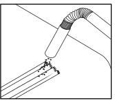
A rivet must be located into each hole and checked that it fully penetrates. If a second skin is encountered, drill second skin then with a centre punch then counter sink the hole to allow clearance for rivet.
