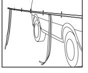
Re-attach crossbars to tracks as shown. Note: Depending on the roof angle the M6 x 16mm screw may be sufficient, otherwise the M6 x 20mm screw and track mount spacer may be required. Tighten security bolt to 3-4Nm.
