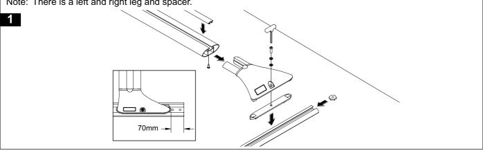
Locate masking tape where tracks are to be positioned. The tracks must be fitted as far apart as possible on the outer edge of the vehicle roof. The track must have full contact with the vehicle roof. Place the crossbar and leg assembly onto the roof. Once location has been decided check on underside of roof for clearance. Ensure crossbars are located as shown.
