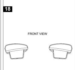
With the Leg/Crossbar units tight and fixed in place the rubber roof trim can be cut and slid in place to cover the exposed areas of the Track at each end. The End Cap is designed to sit over the rubber roof trim after it is cut. Therefore there is a generous tolerance on the measurement of the rubber roof trim.
