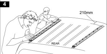
Accurately centre punch all holes before drilling.
