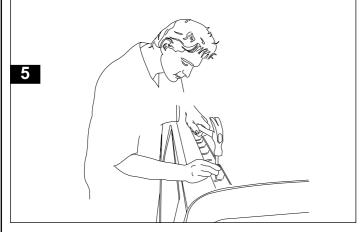
Marked out holes can now be drilled through using a 5mm drill bit and drill stop. Set the drill stop to ensure you don't drill through the roof lining. Use of a drill stop will alleviate the need to remove the hood lining.
