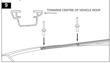
Using either a pneumatic or concertina type rivet gun, rivet the track into place. Make sure all rivets are seated firmly onto the base of the track.
