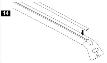
Place the bottom pad over the Dowel Nut Housing then Top Pad. Sit the Leg/Cross bar assembly on the Top Pad. Place the M6 Security Screw and washers through the hole in the Leg as shown and screw into the Dowel Nut. Tightening torque is 3-4Nm. Tighten after positioning both sides equally.
