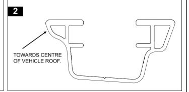
Place the track in the channel and measure from the edge of the windscreen rubber to the front of the track. The use of masking tape will help maintain this measurement while marking out holes for drilling.
