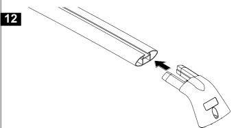
From the underside of the cross bar insert the Phillips head screw.
