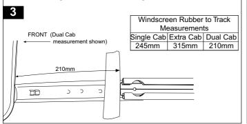
Hold track down tight in roof channel. Mark all holes using a marking pen. Remove the track.
