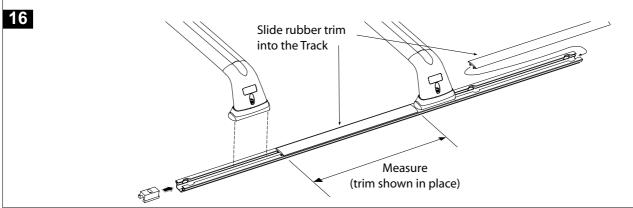
Measure and cut the rubber roof trim and put back in the vehicle roof channel at the front and rear ends of the Track. The front piece needs to be measured so the end of it sits under the windscreen rubber. The measurement and cutting of the rubber roof trim isn't critical since the End Cap will cover it. Recommend using a fine tooth hacksaw because of metal inside the rubber roof trim.
