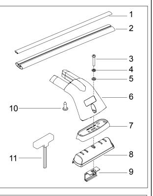
Image: Sports leg into each end of the cross bars. A rubber mallet may be required to knock the leg in place.
