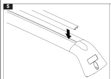
Insert correct length buffer strip into top of crossbar.
