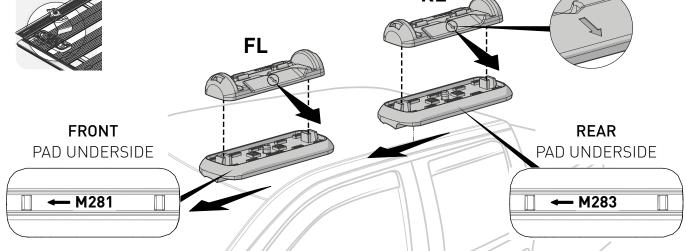
Assemble the **Right Hand Side** legs by facing the pad arrows towards the FRONT of the vehicle and the Foot Plate facing the OUTSIDE of the vehicle.
