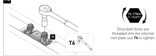
Once both bolts are threaded into the internal
