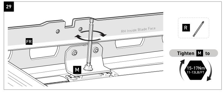
**30 Repeat** Step **29** for all remaining feet: Incrementally tighten the hardware for all six leg locations.
