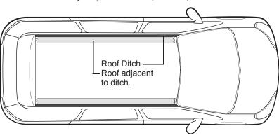
Place the Tracks on the masking tape 240mm from the Trunk Door Jamb. The Track should follow beside the contour of the roof ditch moulding.
