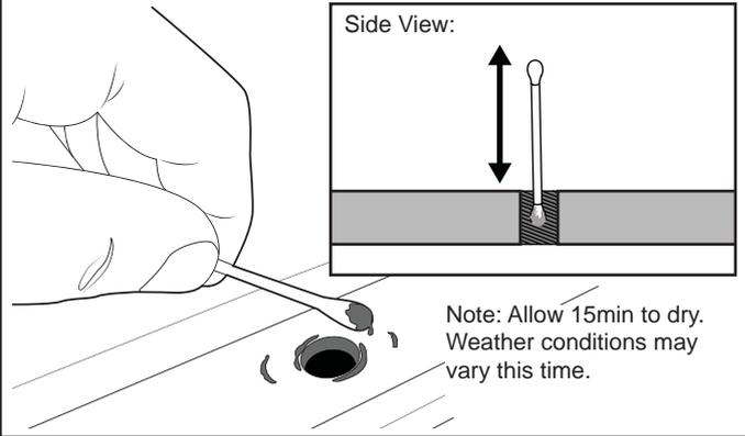
**6** Peel off the one side of backing tape on the Butyl Patches provided. Place these carefully over all holes drilled. Remove the top layer of backing tape as shown.
