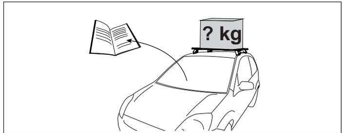
When these roof racks are to be used on a vehicle that is driven off sealed roads, the manufacturer maximum roof load rating (to be found in the vehicles User Manual) should be **divided by 1.5**. Do not forget to subtract the complete crossbar system weight from your maximum carrying capacity.
