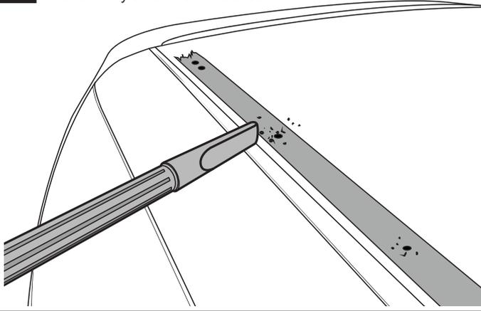
**5** Remove the Masking Tape. Using Cold Galvanising Paint, cover all drilled areas and any exposed body work.
