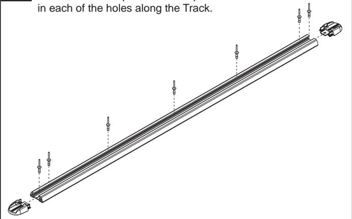
**8** Using either a Pneumatic or Concertina type Rivet Gun (not a small hand gun), rivet the Track into place. Make sure all Rivets are seated firmly onto the base of the Track, place the Rivet Gun onto the Rivet with a Rivet Spacer and gently tap on the back ensures the rivet is seated before compressing. **Check Track alignment carefully before starting. Start at the front and move towards the rear.**
