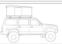
When these roof racks are to be used on a vehicle that is driven off sealed roads, the manufacturer maximum roof load rating (to be found in the vehicles User Manual) should be *divided by 1.5*. Do not forget to subtract the complete crossbar system weight from your maximum carrying capacity.
