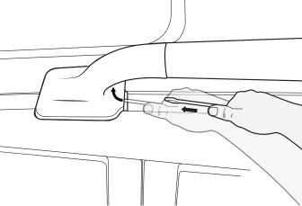
Slide the Screw Driver into the top of the End Cap as shown. Carefully twist the Tool until the Cap pops free.
