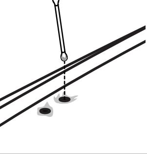
**8** 1: Remove the backing tape from the Butyl Patches. 2: Place them over all holes drilled. Remove the tape from the top of the patches.
