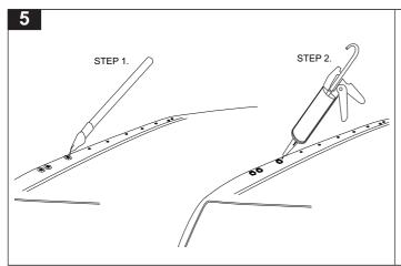
Apply a liberal amount of cold galvanizing solution to the inside and surrounds of all holes. Allow cold galvanizing solution to dry, three to four minutes, then apply a liberal amount of Selleys Butyl Mastic in and around each hole.
