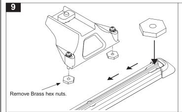
Unscrew the brass hex nuts from the RLTP leg. Place the hex nuts off each RLTP leg into the large cut out at Rear of track and slide along to desired position. The legs will be fitted in place after the cross bars are attached.
