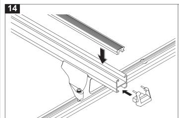
Insert the cross bar rubber buffer strip into the top of the cross bar. Insert the end caps into the ends of the cross bar, a rubber mallet may be required to fit the end caps.
