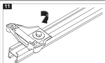
Finger tighten the leg attachment bolt so that the channel nut turns to locate across the cross bar. Leave loose enough so the cross bar can slide along the leg. The legs will require final adjustment and tightening later.
