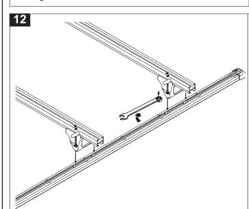
Locate the RLTP legs onto the tracks then fasten M6 security screws into the brass hex nuts. Leave loose for adjusting the legs and cross bars along the Track extrusion.
