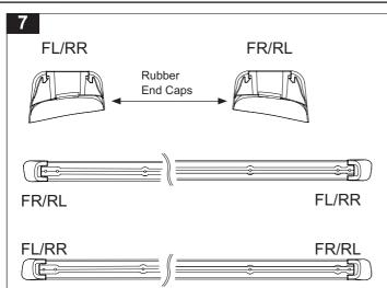
Fit the rubber end caps to the tracks. The end caps are marked on the underside to denote thier positon.
