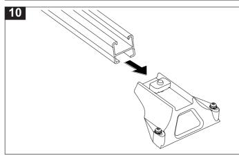
Slide the cross bar onto the leg and locate with the M10 channel nut. Leave untensioned at this stage.
