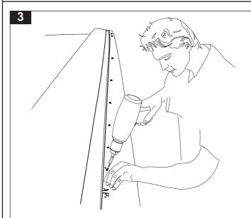
All ten holes can now be drilled through. A drill stop is recommended to prevent drilling through the hood lining on the inside. **Make sure that when drilling you hold the drill perpendicular to the roof angle.** The roof skin is approx. 1-2mm thick.
