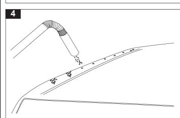
Use a vacuum to remove swarf to eliminate scratching. Wipe clean the installation area of the roof.
