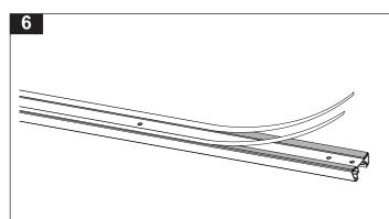
Peel the white backing strip off the track foam tape.
