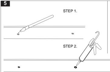
**STEP 1.** Apply a liberal amount of cold galvanizing solution to the inside and surrounds of the drilled holes only. Allow cold galvanizing solution to touch dry, ten minutes or so.
