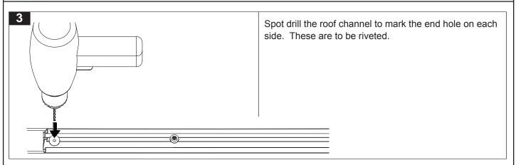
Remove the screws and track. Drill through the roof in one spot each side. Use a vacuum cleaner to remove swarf from the roof. This will minimise swarf entering the hole and avoid scratching. Wipe after with a rag.
