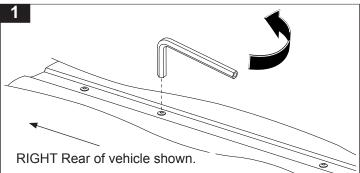
Using the 5mm allen key supplied remove all 8 screws in the roof channel.
