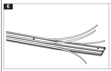
Peel the four white backing strips off the foam tape on each track.
