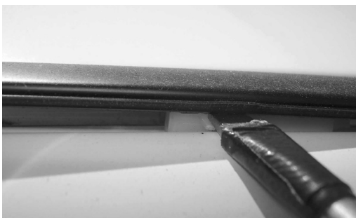
LIFT TRIM FROM OUTSIDE EDGE OF ROOF.
