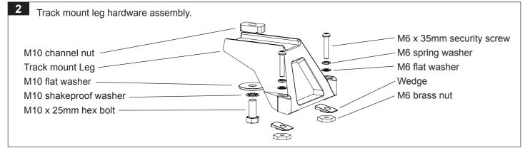
3 Insert legs into each end of the crossbars. Check that the channel nut is located across the bar as shown in Figure 4a. Do not tighten at this stage.
