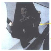
Assemble crossbar to the support legs with one pair of leg height spacers for the AU Wagon. Leave legs loose for adjustment.
