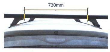
Assemble the support legs onto the crossbars for both the front and the rear bar.
