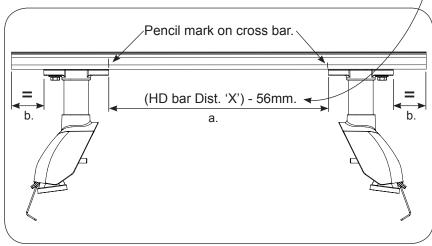
Channel nuts must fully locate across the cross bar when tight.
