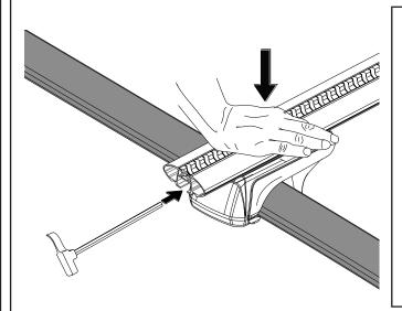
With Torque Key inserted, turn clockwise until handle straightens as below. This indicates 4-5 Nm. More pressure may be required in extreme climates.
