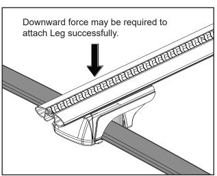
Fasten each Leg alternately using the Allen Key provided to 4-5Nm. Donward force may be required on top of the Crossbar Leg as shown.
