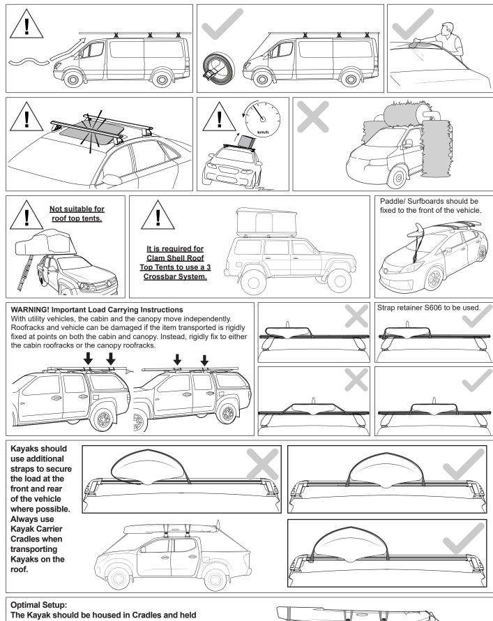
The Kayak should be housed in Cradles and held in place with tension straps.
