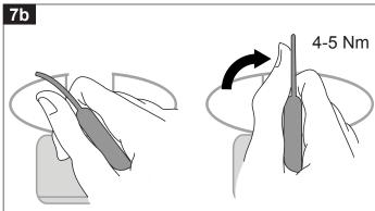
With Torque Key inserted, turn clockwise until handle straightens out as shown above. This indicates 4-5 Nm. More pressure may be required in extreme climates.
