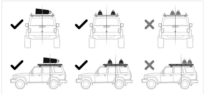
Distribute loads evenly and laterally/longitudinally as low as possible over the span.
