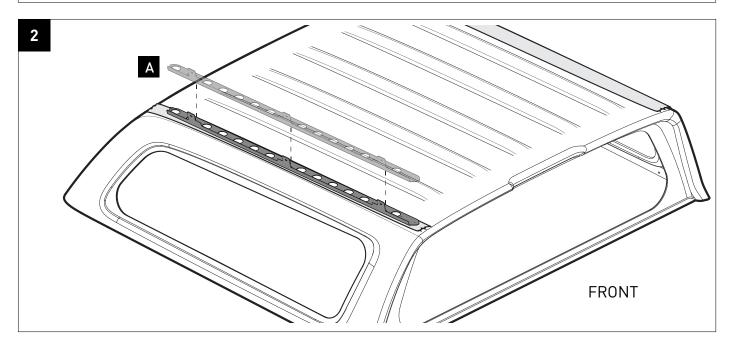
3 Align to a flat area near the edge or next to a reinforcing 'rib' near the edge (strongest area of roof)
