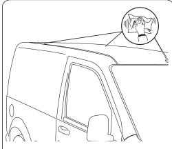
Wash vehicle roof prior to installation. Please read through instructions before fitting the racks to your vehicle.
