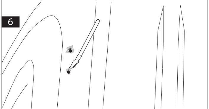
Apply Silicone or Butyl Mastic liberally over and around each drilled hole.
