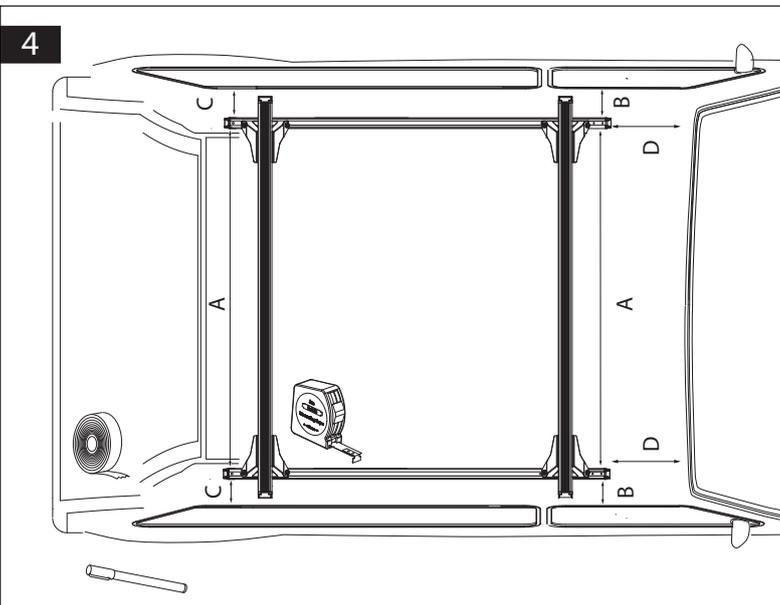
Place assembled crossbars and tracks on top of the vehicles rooftop as shown. Ensure system is adjusted so all measurements are even.
