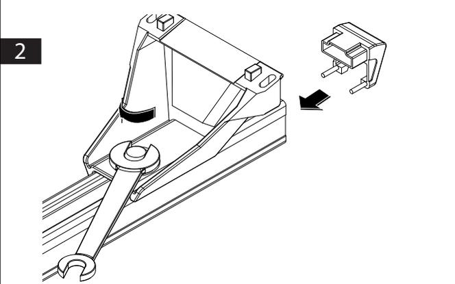
Slide the eight M6 brass hex nuts into the track as shown. Two brass nuts to each end. Place each assembled crossbar onto the track 50mm from the track end to the closest edge of the track mount leg. Place a M6 spring washer a M6 x 12.5mm flat washer and a M6 x 35mm security bolt into each leg hole. Fasten the leg to the track.
