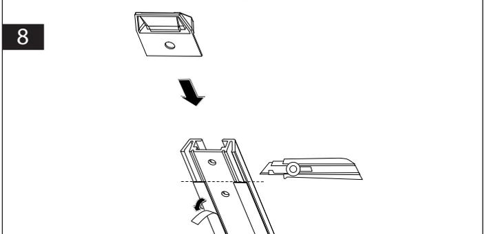
Place the track carefully onto the vehicles rooftop. Place a 5mm Rivet in each hole to align the track. Use a Pop Rivet Gun to fix the track to the rooftop. Repeat process 5 - 9 for the track on the opposite side of the vehicle.
