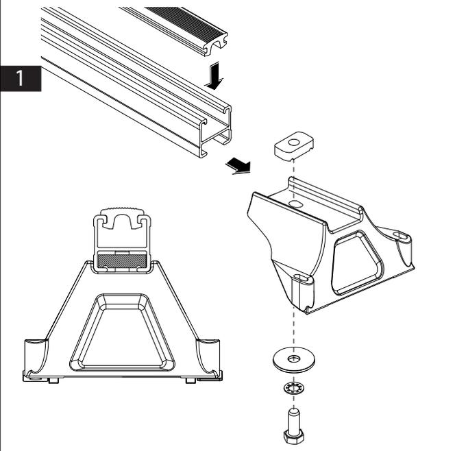
Tighten the leg to the crossbar so it can slide for adjustment. Place two end caps on each crossbar.
