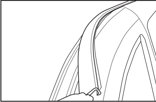
Lift front of the trim from outside edge of roof. Twist outwards to unhook as shown in the diagrams.
