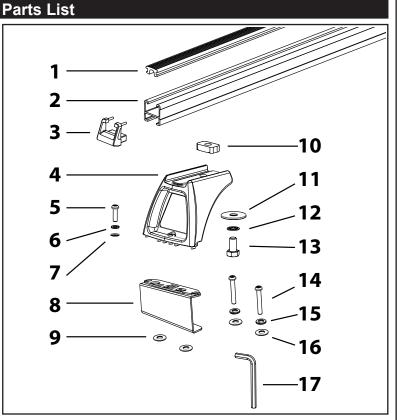
Tools needed: Flat blade screwdriver, Phillips head screwdriver, Rubber mallet, Socket wrench & 13mm socket.
