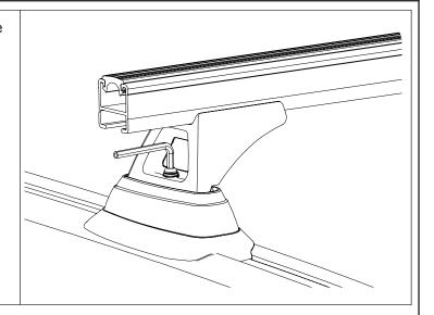
Adjust all cross bars to achieve equal over hang. Tighten the M10 cross bar attachment bolts.
