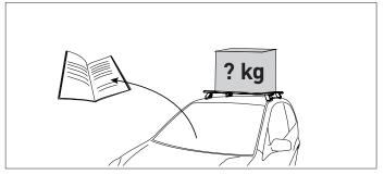
The handling characteristics of the vehicle changes when a load is transported on the roof. Exercise extreme care when transporting wind-resistant loads. Special consideration must be taken when cornering and braking.
