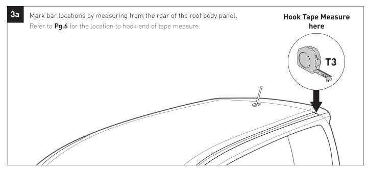
One person to hold the tape end down from the end of The other person marks the centre of the ditch for the bar locations on both sides of the vehicle. the roof panel sheet metal. **T7** See Step 3b 3b **3 CROSS BAR CONFIGURATION** Use the below dimensions to mark the cross bar mounting points. 1835 784 283 R ⊦ Use N or O to align the V-cut indicator from the jig/bracket to mark hole centres. **T7** Ν 0 Inside edge of **ENTRE OF** ditch
