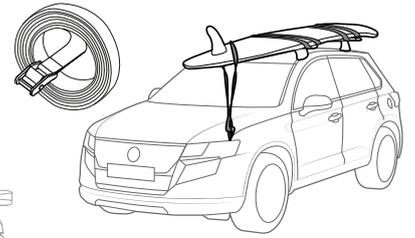
Use only non-stretch fastening ropes or straps to attach cargo to roof racks
