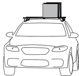
$$\begin{matrix} 75\text{kg}/165\text{lbs} \\ \text{load rating} \\ \text{(Urban road)} \end{matrix} = \begin{matrix} 50\text{kg}/110\text{lbs} \\ \text{load rating} \\ \text{(off road)} \end{matrix}$$
