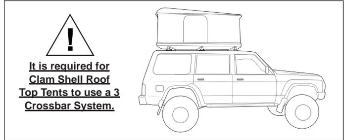
When these roof racks are to be used on a vehicle that is driven off sealed roads, the manufacturer maximum roof load rating (to be found in the vehicles User Manual) should be **divided by a factor of 1.5**. Do not forget to subtract 5kg from your maximum carrying capacity due to the weight of the crossbars and legs.
