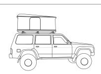
When vehicle is driven off sealed roads, the maximum roof rack load rating should be divided by 1.5. Do not forget to subtract 5kg from your maximum carrying capacity due to the weight of the crossbars and legs.
