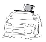
WARNING: Cabin and canopy move independently on utility vehicles. Rigidly fix items to either the cabin roofracks or the canopy roofracks, as fixing on both simulaenously will cause damage.
