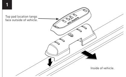
The four top and bottom pads are identical. Diagram shows the correct orientation of top and bottom pad.
