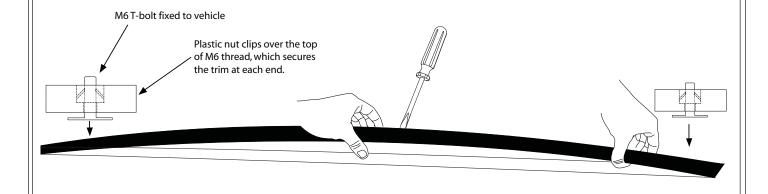
The roof trim has to be cut to the sizes shown so that it will sit neatly under and be held in by the edge of the MDX roof pads when they are screwed into position. A hacksaw is recommended to cut the trim. 120mm of trim in two spots has to be removed from each side. While the trim is out wipe out any dirt to give the pads a clean surface to sit on.
