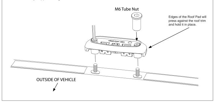
Fit crossbars to pads as be corresponding instructions. When the roof crossbars and legs are removed the roof pads can be covered for protection with the mounting pad cover plates.
