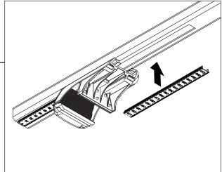
2 Install the crossbar to the vehicle as per the corresponding leg kit instructions. Install end caps as shown.
