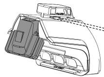
Note the gap in the clamp and the crossbar will slide into. SX044 shown as example only.
