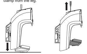
Use the tube nut from SX044 and install the new clamps as shown. You may have to apply pressure to the assembly skewer to seat it correctly back in the leg.
