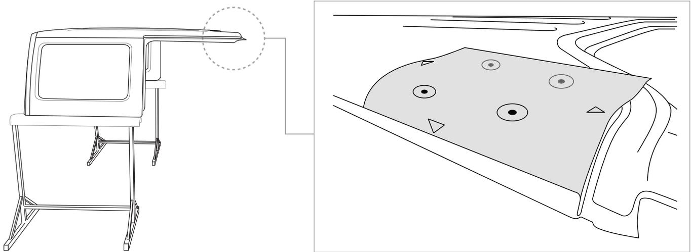
**8b** With the Front Bracket Template placed onto the Hard Top, align as shown and spot mark.
