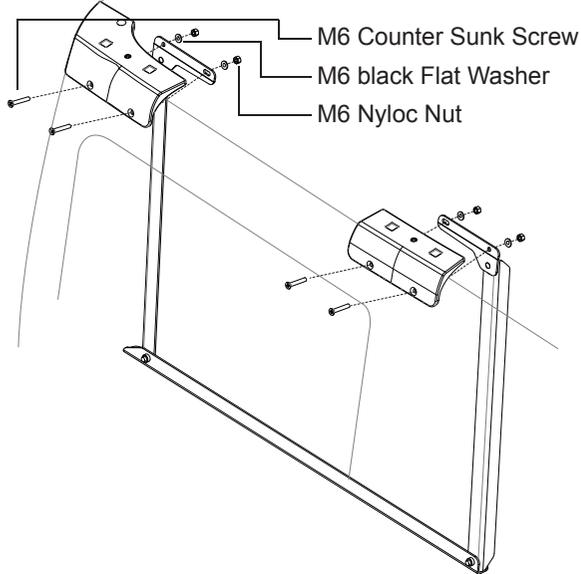
2. Hold Nyloc Nut with a spanner, allowing the bracket to be tightened from the outside.
