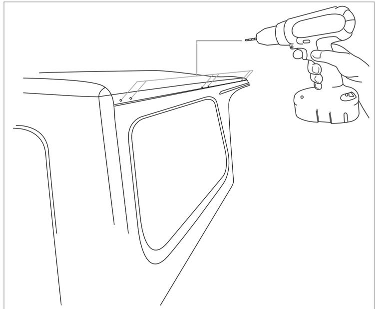
**10** Using a 6.5mm (1/4") drill bit, drill out the **REAR and MIDDLE** spot drilled sections on the Hard Top.
