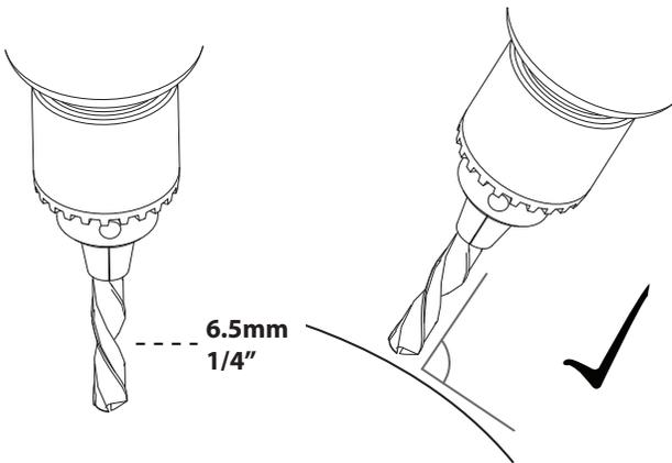
**11 FRONT HOLES ONLY:** Using a 6-18mm step drill bit, open out the front spot holes as shown.
