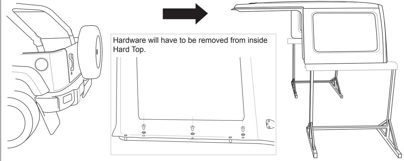
**2a** Assemble the Support Struts as shown. Finger tighten. Check part ID to make left and right side supports.
