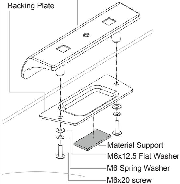
Tighten Backing Plate to the Front Bracket from the inside of the Hard Top. Max Torque 4-5Nm/ 3-4lbs/ft.
