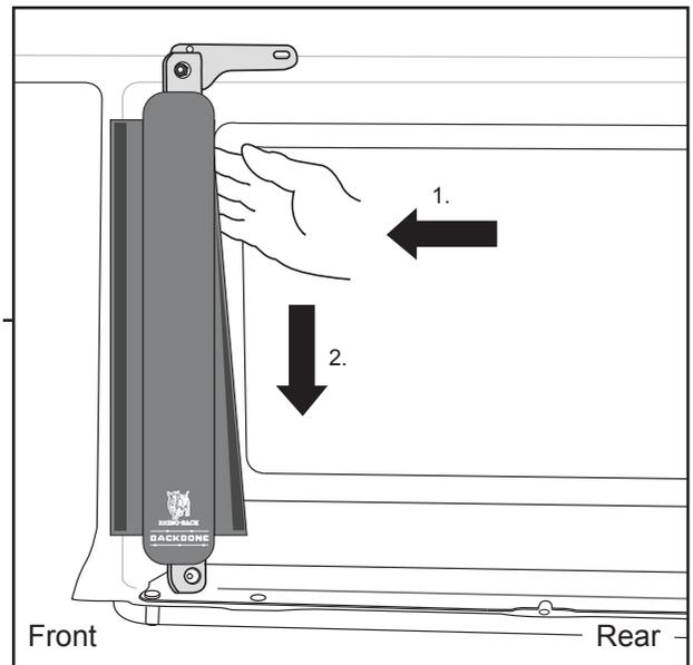
**30** Hold the looped velcro in place (as in previous step). 1- Push the remaining velcro around the back of the Backbone bracket. 2- Moving down the pad, push all of the velcro into place. Be sure velcro is secure before driving.
