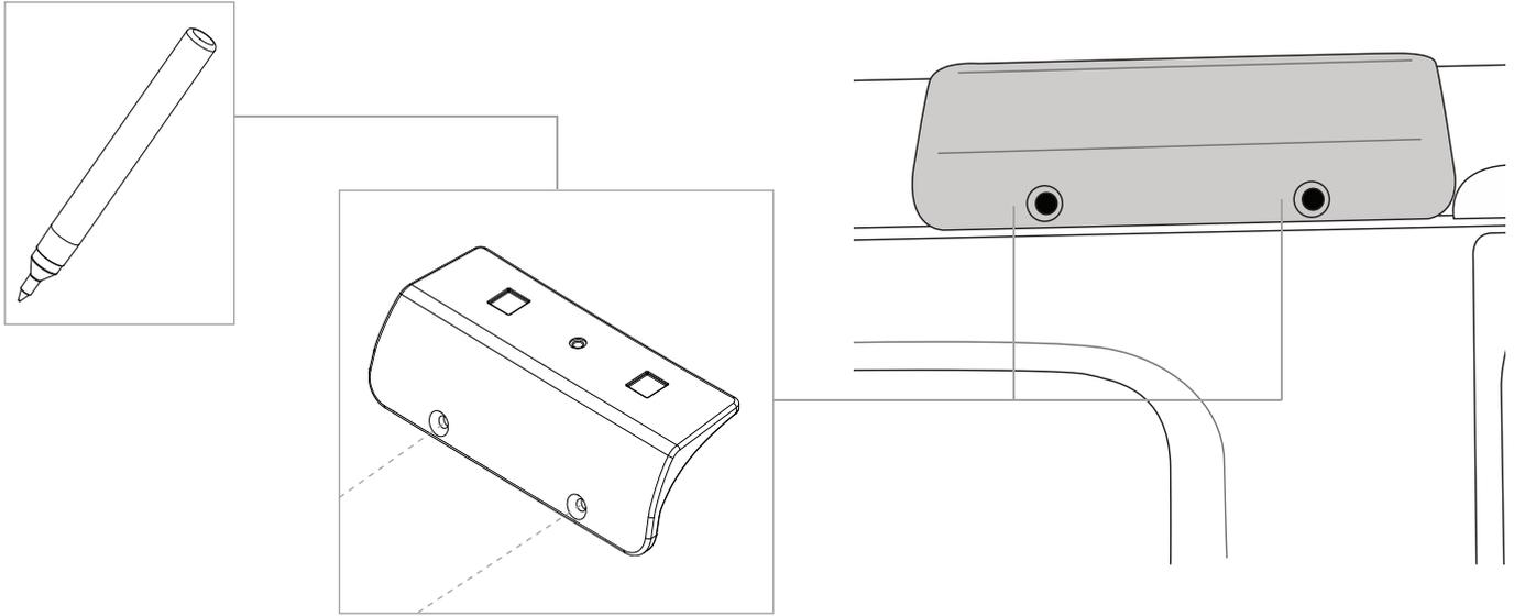
**8a** Place the Front Bracket Template onto the Hard top as shown (template as suppliment).
