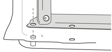
B. The Support Strut will slot onto the Hard Top studs as shown.
