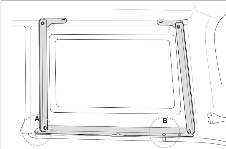
A. The Support Strut will slot onto the Hard Top studs as shown.
