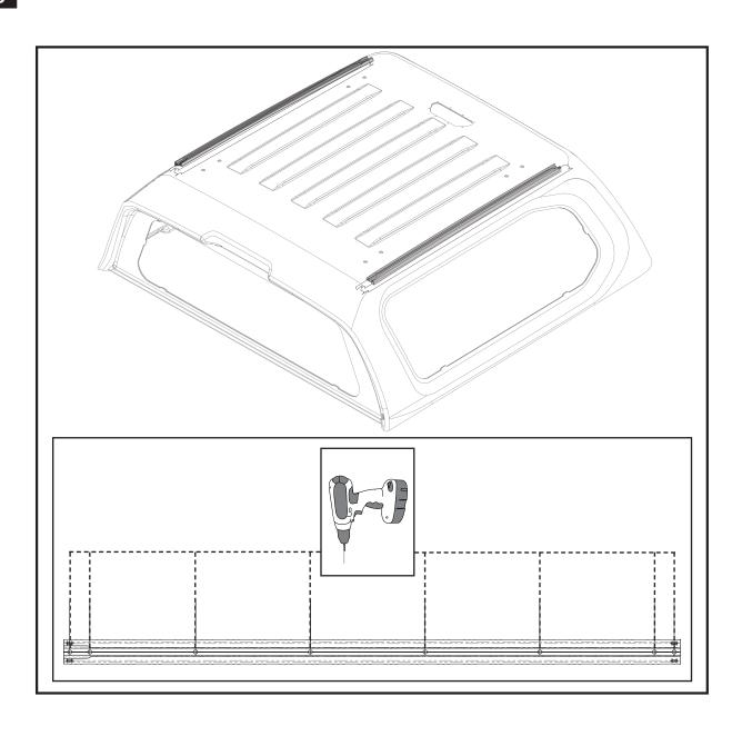
Using a sharp  $\emptyset$ 6.5mm bit, hold the drill perpendicular to the surface of the canopy, apply minimal pressure and proceed to drill. Make sure both the inner and outer skins are drilled through. Repeat process with an  $\emptyset$ 8mm bit. Remove any swarf with a vacuum.
