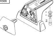
\*Fix the Quick Mount Spacer to the Leg using the hardware in the leg kit. The bolts found in the spacer kit will replace the original in the leg kit.
