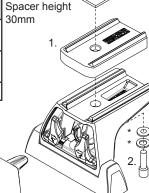
\*Fix the Quick Mount Spacer to the Leg using the hardware in the leg kit. The bolts found in the spacer kit will replace the original in the leg kit.
