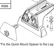
using the hardware in the leg kit. The bolts found in the spacer kit will replace the original in the leg kit.
