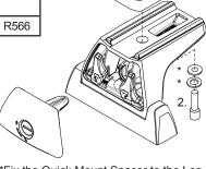
\*Fix the Quick Mount Spacer to the Leg using the hardware in the leg kit. The bolts found in the spacer kit will replace the original in the leg kit.
