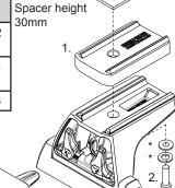
\*Fix the Quick Mount Spacer to the Leg using the hardware in the leg kit. The bolts found in the spacer kit will replace the original in the leg kit.
