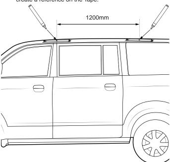
Place a Bracket into the Ditch with the centre hole of the Bracket in line with the reference made previous. The Bracket will sit at the front of the Ditch partially on top of the body fill as shown.
