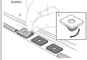
Press the Ditch Brackets into position over the drilled holes. Using a Pneumatic Rivet Gun, fix the Brackets in place with Rivets provided. Be sure Brackets are aligned correctly.
