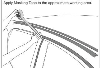
2 Starting from the Door Jamb of the vehicle, measure out the references below. Place a strip of Tape at these points. Create a reference on the Tape at these measurements with a Marker.
