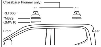
\*NOTE: M829 will sit on top of the installed Bracket. The Gasket will cover exposed areas of the Bracket and Ditch Fill.
