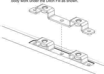
Using a 4.85mm Drill Bit with a Drill Stop (set to 5mm), spot mark the three rivet holes in the Bracket. Do not drill through the roof at this stage.
