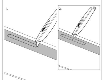
5 Starting in the centre of previously cut Fill and using a Scrape, remove the cut sections of Ditch Fill. Remove the Masking Tape on the Fill.
