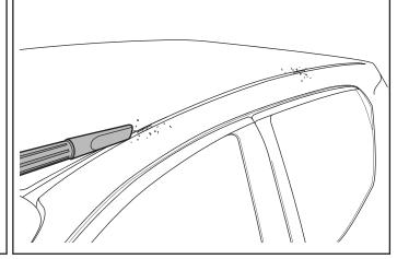
Apply Cold Galvanising Paint. Make sure to spread around drilled holes as well as inside. A layer should be put over all exposed bodywork. Allow 10min to dry. Weather conditions may alter drying time.
