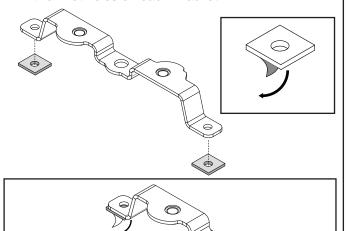
Refer Step 2 for correct orientation: Place Ditch Brackets into position. 1: Install M8 Hardware to fasten the Bracket. 2: Using a Pneumatic Rivet Gun, fix the Brackets in place with Rivets provided.
