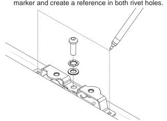
Remove the Bracket. Use a 5mm Drill Bit with a Drill Stop set to 8-9mm. Open up all marked rivet holes.
