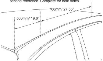
Place the QMFK Bracket centred onto these points previously made. Mark out the rivet holes onto the ditch. Be sure Brackets are parallel.
