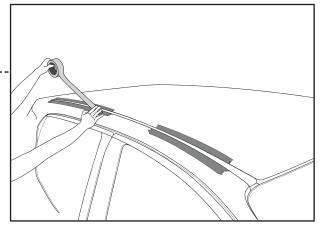
Starting from the Door Jamb of the vehicle, measure out the references below. With a Marker, indicate these points onto the Tape next to the Ditch Mould.
