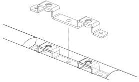
Top View: Front Bracket. Bracket must pivot 5mm in toward the centre of the vehicle.
