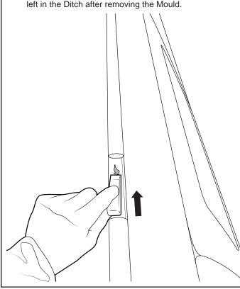
Replace the Brackets into the Ditch. The leading edge of the **Front Bracket must pivot 5mm in toward the centre of the vehicle.** This will ensure all Brackets are parallel in the Ditch.
