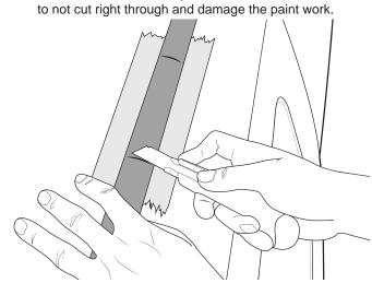
1: Hook a hand inside the Mould and pull towards the outside of the vehicle. 2: With assistance, cut out the areas of Mould marked out previous. Use extreme caution with cutters, ensuring the tool doesn't touch the paintwork.
