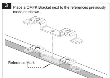
Mark either end of the Bracket onto the Ditch Mould.
